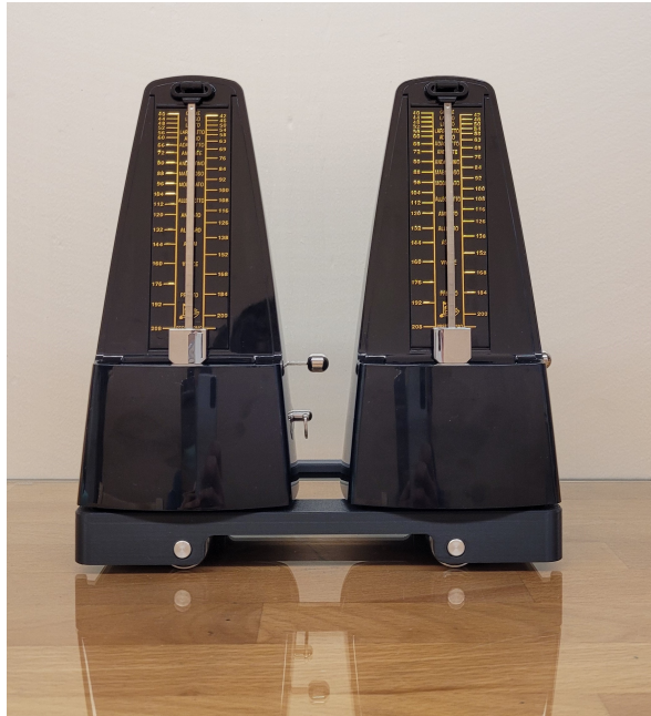
Figure 4: Metronomes on a common sliding base.
