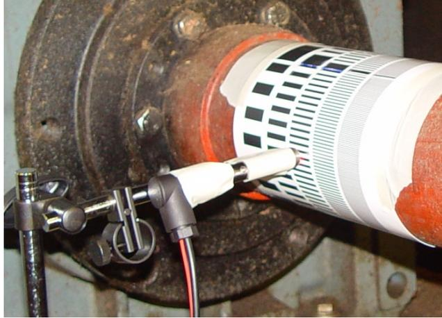
Figure 10: The digital encoder and the optical sensors' setup for the pendulum shaft-angle measurement
