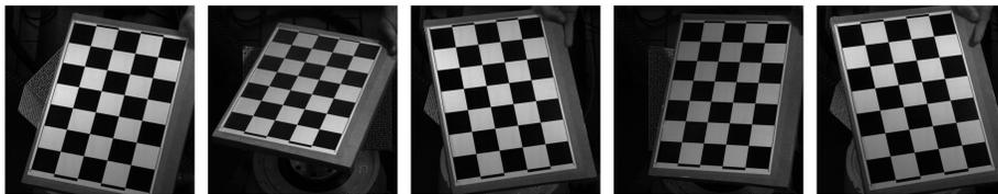
Figure 6: Five images of the checkerboard pattern, used in intrinsic parameter estimation.
