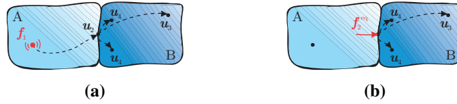
Fig. 1: Source characterization using in-situ TPA: a) assembly under operation; b) set of equivalent forces replicating the operational response.
