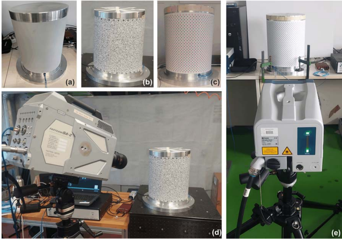
Fig. 2: (a) Flanged cylinder, (b) cylinder with the speckled surface, (c) cylinder with the circular markers, (d) optical camera measurement, (e) laser vibrometer measurement.
