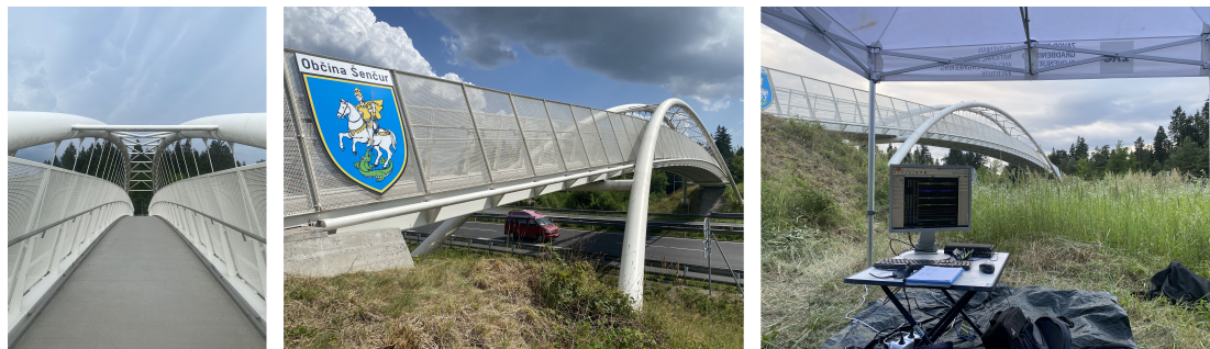
Fig. 1: Lateral and side view of the pedestrian and cycling bridge with data acquisition station during experimental campaign.
