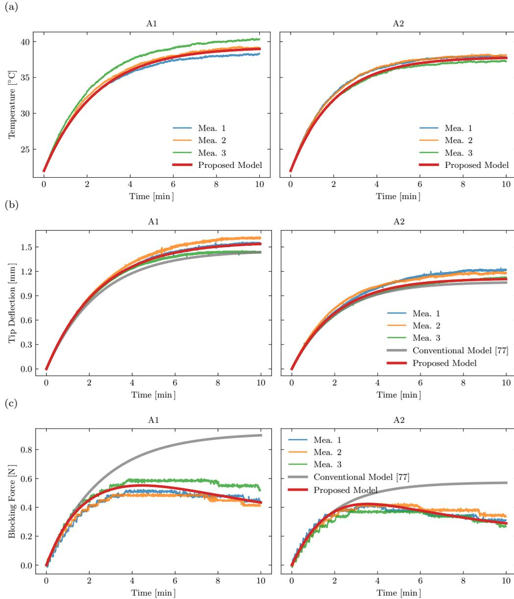
Figure 7: Measured and predicted responses of A1 (left) and A2 (right) electrothermal actuators: (a) average temperature on the outer surface of M1, comparing measurements (Mea.) with the proposed analytical model; (b) tip deflection, comparing measurements (Mea.), the conventional model [77] (gray), and the proposed model (red); and (c) blocking force, also compared among measurements (Mea.), the conventional model (gray), and the proposed model (red).
