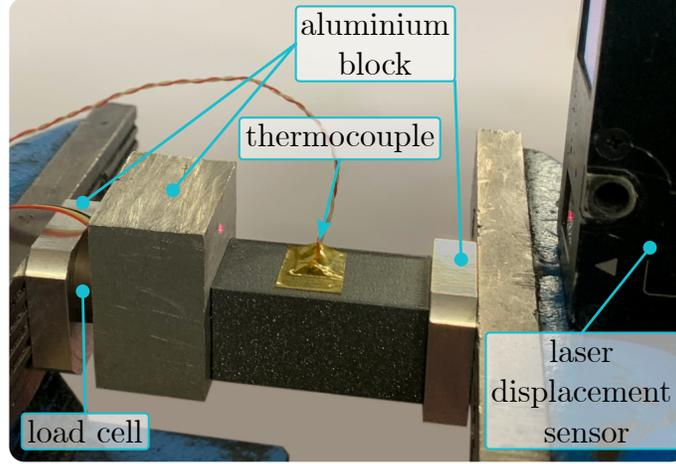
Figure B.10: Experimental setup for measuring the relaxation modulus of 3D-printed rectangular samples. A load cell records the compressive force, and a laser displacement sensor tracks the step deformation. A thermocouple positioned on the sample monitors temperature, while aluminum blocks ensure uniform contact with the compression jaws.
