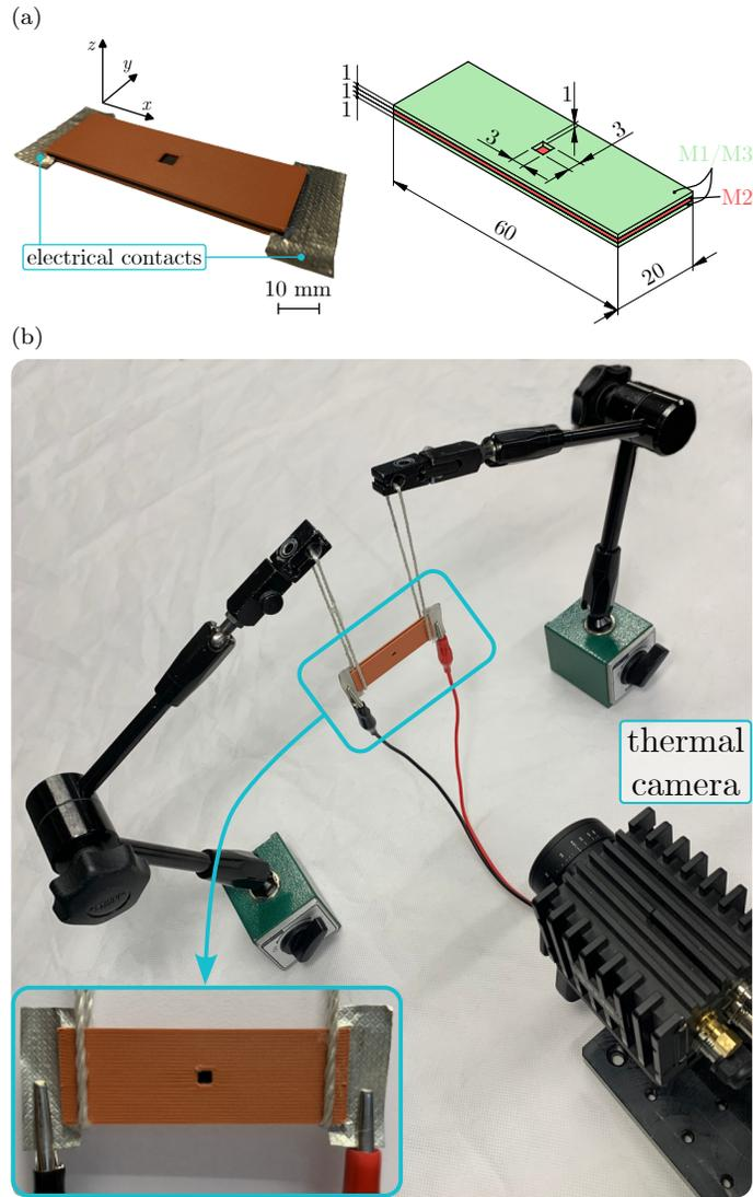
Figure B.12: (a) Rectangular, three-layer sample used for thermal conductivity and specific heat measurements, featuring a small central cavity to monitor temperature distribution. (b) Experimental setup in which the sample is suspended by two ropes and heated via a step voltage, while a thermal camera records surface temperatures for both transient and steady-state analyses.
