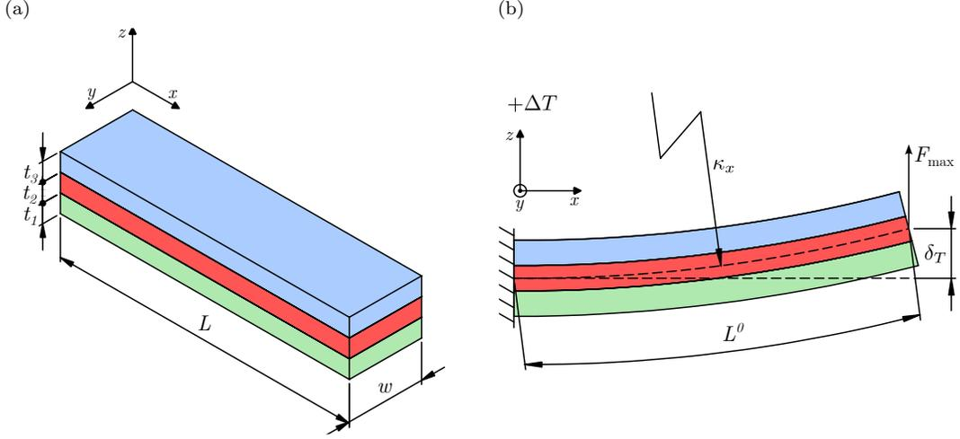
Figure 2: (a) Schematic of the three-layer bimorph actuator in its initial state, with layers arranged from bottom to top as M1 (high CTE), M2 (heater), and M3 (low CTE). (b) Actuated state when a voltage is applied to M2, causing a temperature increase. The resulting thermal expansion mismatch induces a mid-plane curvature  $\kappa_x$ , leading to a tip deflection  $\delta_T$  and a blocking force  $F_{\max}$ .
