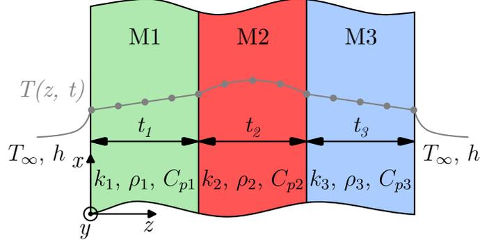
Figure 5: One-dimensional thermal model of the three-layer actuator, assuming uniform properties in the  $x$ - $y$  plane and internal heat generation in the middle layer. Each layer is assigned thermal properties along the  $z$ -axis, with convective boundary conditions applied at the outer surfaces.
