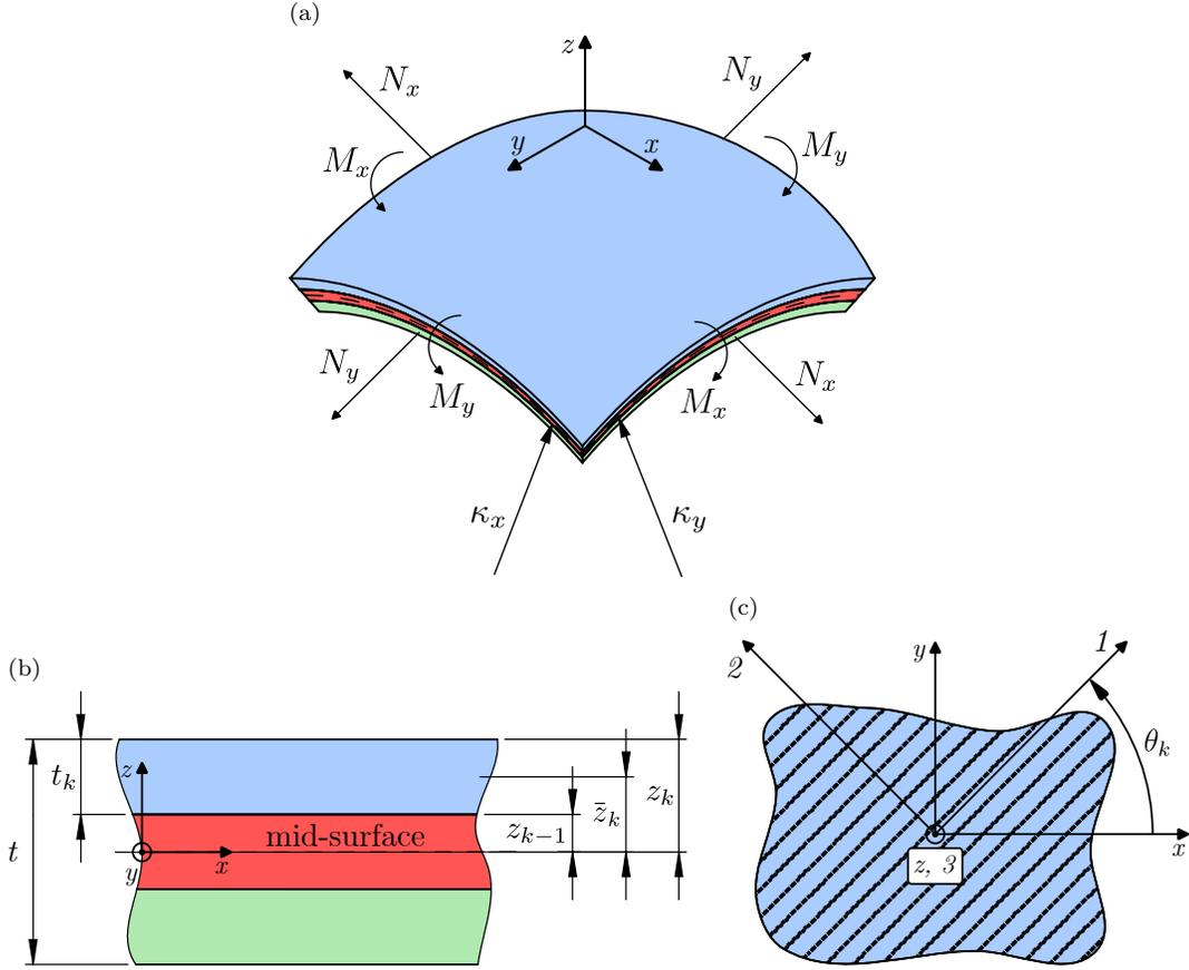
Figure A.9: (a) Schematic illustration of a laminate with mid-surface curvatures  $\{\kappa\}$  and mechanical loads and moments ( $\{\mathbf{N}\}$  and  $\{\mathbf{M}\}$ ). (b) Cross-sectional view showing the total thickness  $t$ , divided among individual laminae. (c) Fiber orientation in each lamina, with principal material axes defined relative to the  $x$ -axis by the angle  $\theta_k$ .
