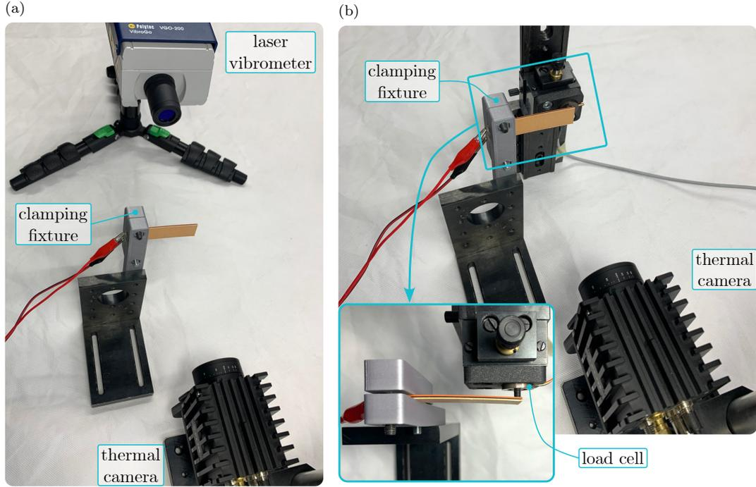
Figure 6: (a) Experimental setup for measuring the tip deflection of the 3D-printed actuator using a laser vibrometer. The actuator is clamped at one end to provide a fixed boundary, and a thermal camera monitors the surface temperature. (b) Setup for blocking force measurement, with a load cell positioned at the actuator tip. In both experiments, a step voltage is applied to the actuator.
