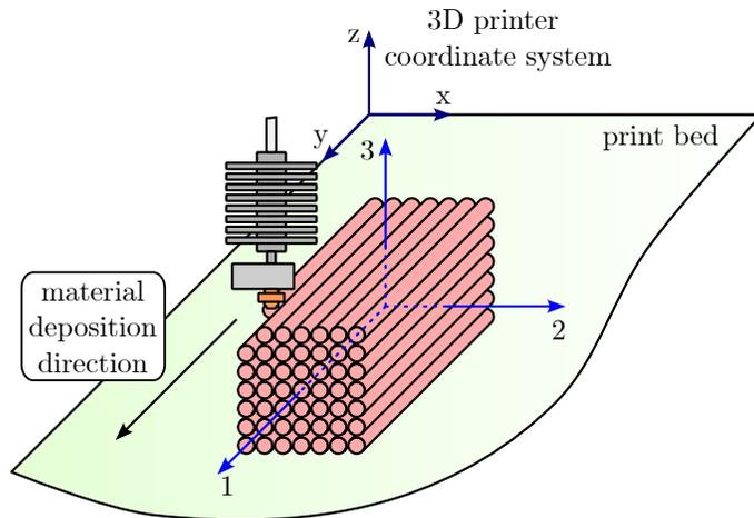
Figure 1: Schematic of a unidirectional 3D-printed structure illustrating its principal material coordinate system: axis 1 is aligned with the print direction, axis 2 lies in-plane and perpendicular to the print direction, and axis 3 is normal to the printed layers, representing orthotropic material behavior.
