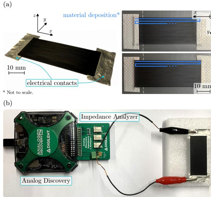
Figure B.11: (a) Rectangular 3D-printed sample (dimensions vary) used to measure electrical resistivity, with conductive tape applied at both ends to ensure reliable electrical contacts. (b) Experimental setup for resistance measurements, with an impedance analyzer connected to the sample via crocodile clips under a constant DC voltage.
