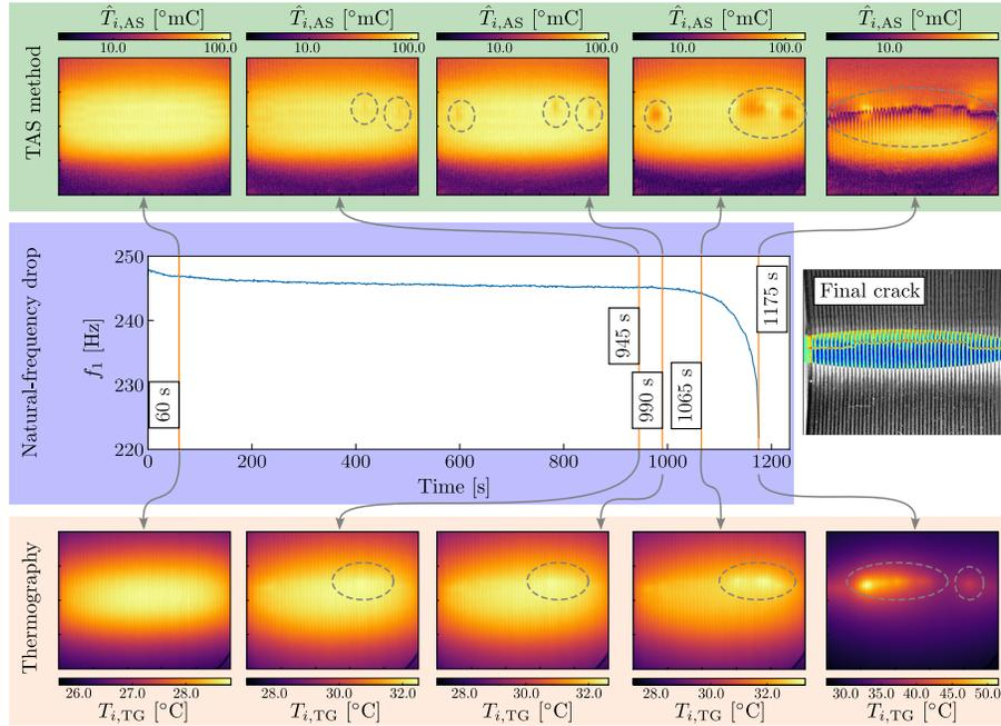
Figure 7: Crack identification of specimen no. 2 (3D printed in  $x$  direction) during vibration-fatigue testing using the TAS method (upper section) and Thermography method (bottom section) in reference to the drop of the specimen's natural frequency and a final crack in the middle section.
