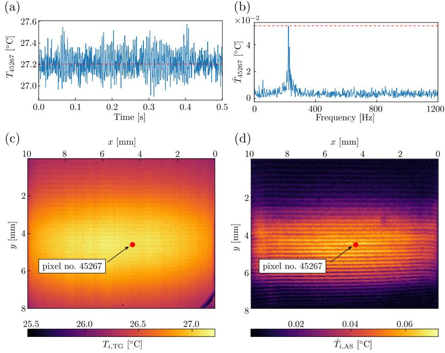
Figure 4: Temperature response of the specimen no. 1; (a) time waveform for pixel no. 45267, (b) amplitude spectrum for pixel no. 45267, (c) heatmap of observed area obtained with Thermography method and (d) with TAS method.
