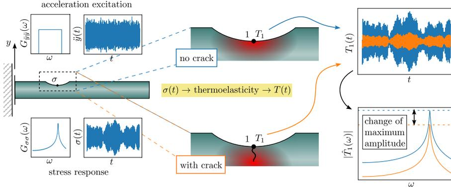
Figure 1: Crack detection concept: the temperature signal during the vibration test due to the thermoelastic effect and its changes in the presence of a crack.
