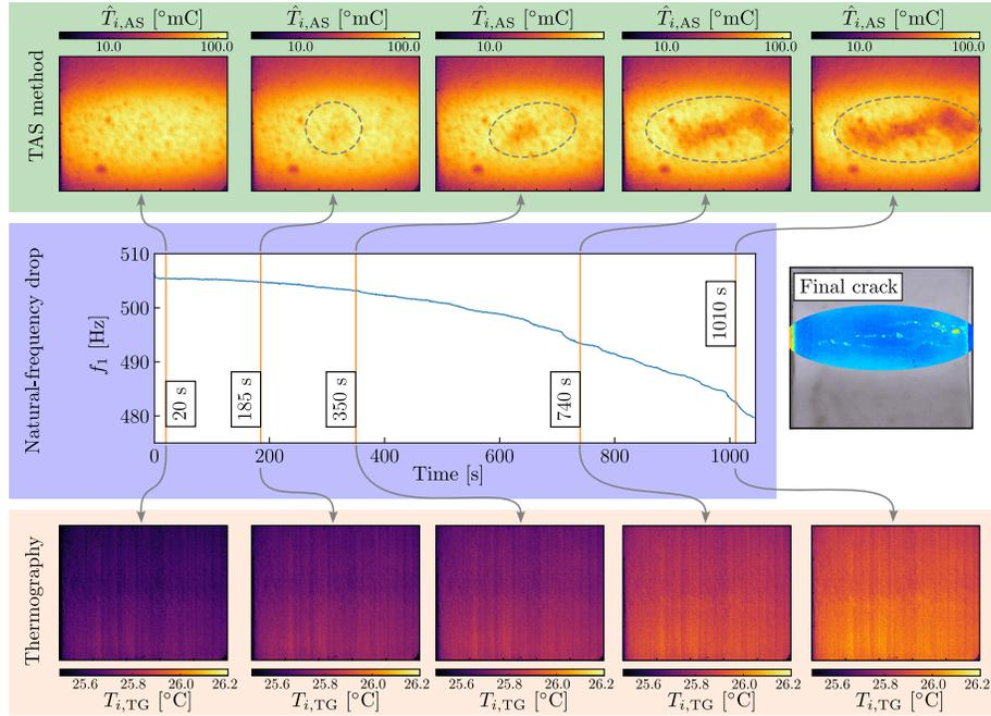
Figure 8: Crack identification of specimen no. 3 (aluminum with prepared surface) during vibration-fatigue testing using the TAS method (upper section) and Thermography method (bottom section) in reference to the drop of the specimen’s natural frequency and a final crack in the middle section.
