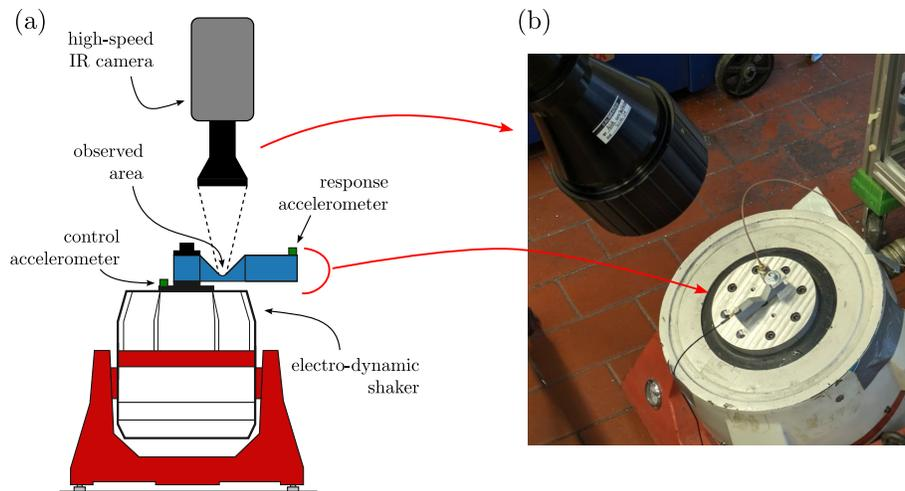
Figure 3: Experimental setup; (a) a schematic representation with an electrodynamic shaker, mounted specimen and a high-speed IR camera, (b) an actual setup.
