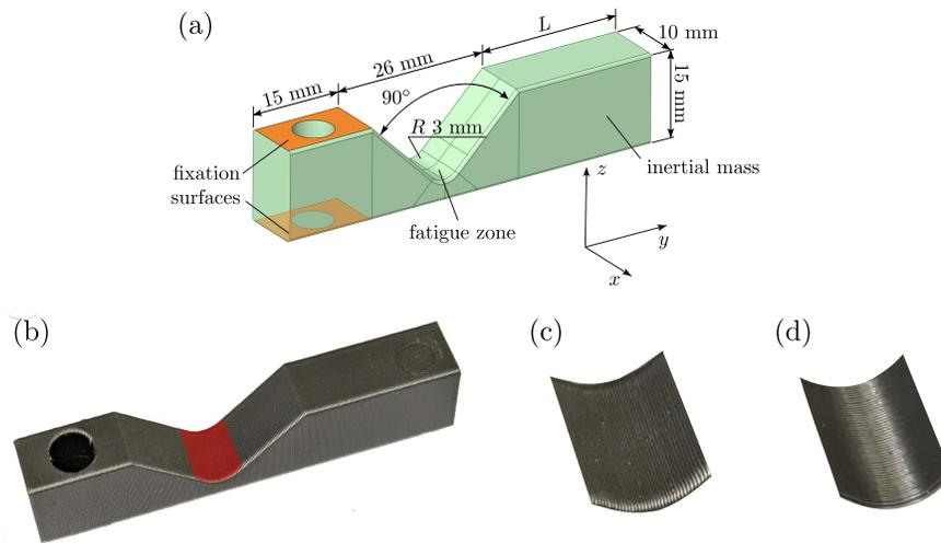
Figure 2: Specimen design; (a) specimen geometry with adopted coordinate system, (b) manufactured specimen with denoted observed fatigue zone, (c) zoomed-in fatigue zone for specimen 3D-printed in  $y$  direction and (d) in  $x$  direction.
