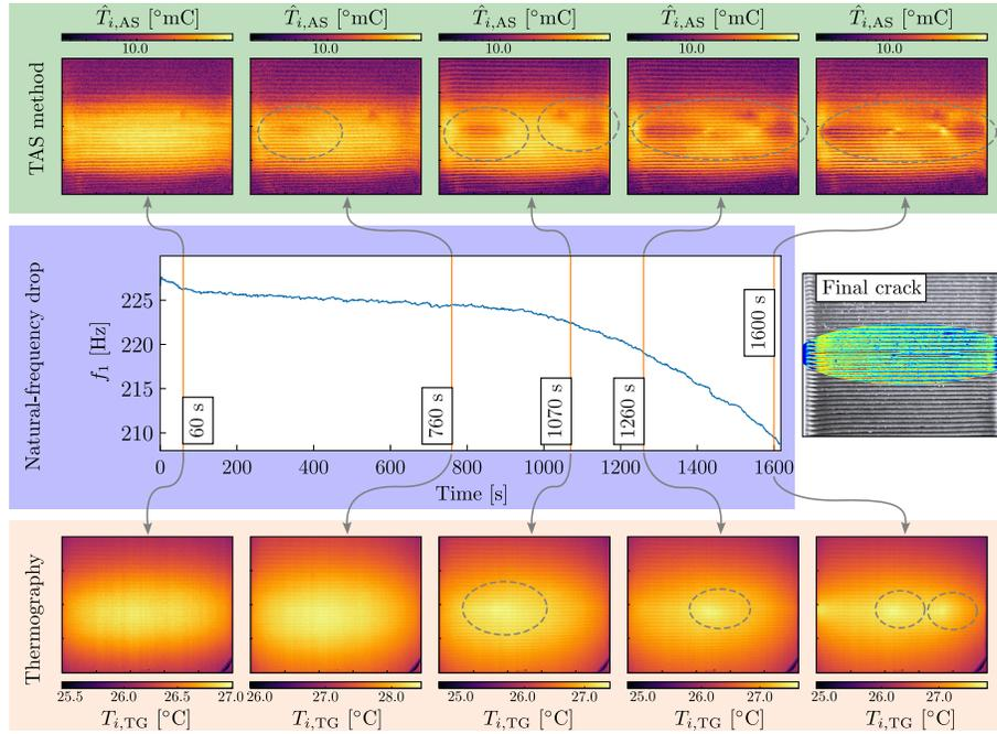
Figure 6: Crack identification of specimen no. 1 (3D printed in  $y$  direction) during vibration-fatigue testing using the TAS method (upper section) and Thermography method (bottom section) in reference to the drop of the specimen's natural frequency and a final crack in the middle section.
