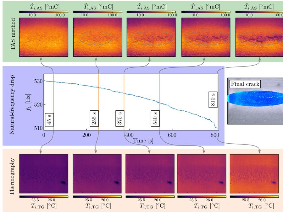
Figure 9: Crack identification of specimen no. 4 (aluminum with surface from water-jet cutting) during vibration-fatigue testing using the TAS method (upper section) and Thermography method (bottom section) in reference to the drop of the specimen’s natural frequency and a final crack in the middle section.
