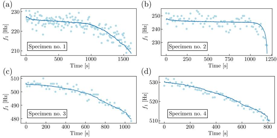
Figure 5: Comparison between (—) specimens' identified natural frequencies with a response accelerometer and (●) averaged frequency of  $\hat{T}_{i,AS}$ , graphs (a) - (d) refer to specimens no. 1 - no. 4, respectively.
