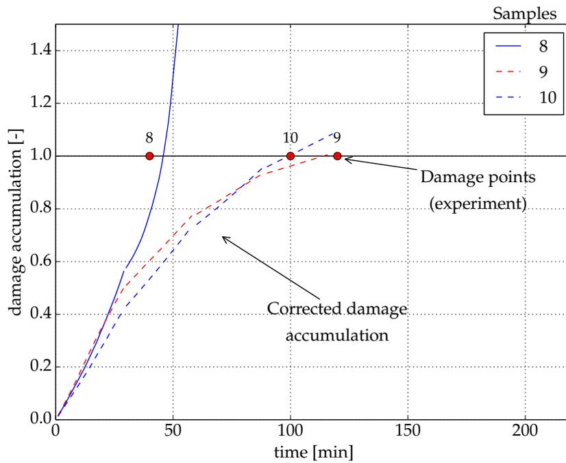
Figure 8: Corrected Damage Accumulation for Different Correction Factor  $R$
