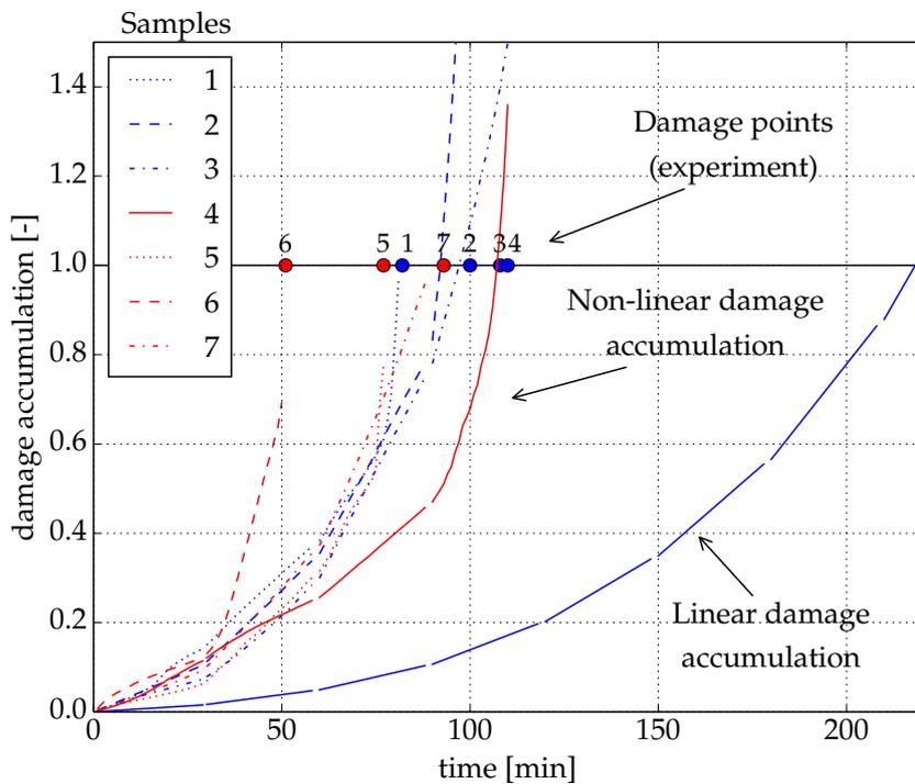
Figure 6: Linear and Corrected Damage Accumulation ( $R=160$ )
