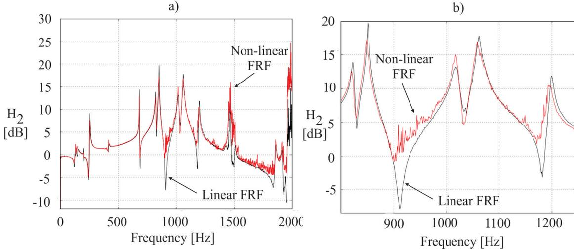
Figure 1: Linear and Non-linear FRFs; a) Whole scale b) Detail
