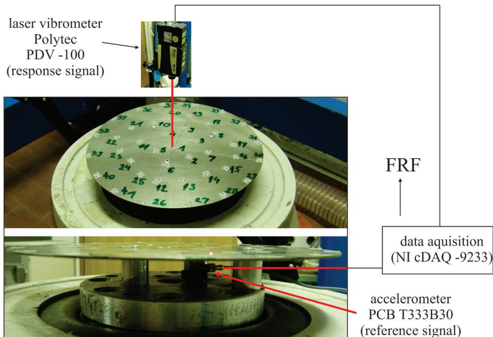
Figure 4: Electro-Dynamic Shaker and the Experimental Setup
