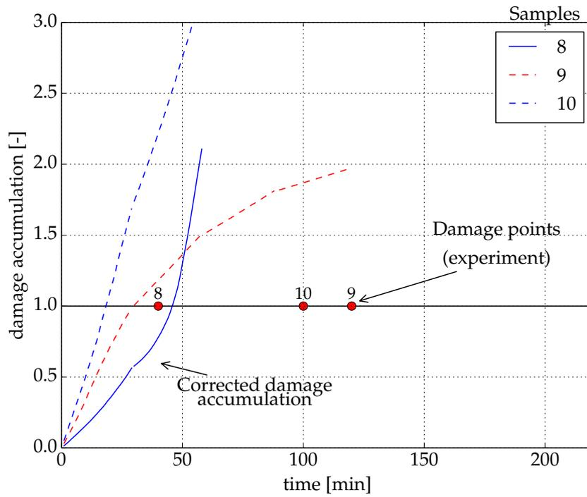
Figure 7: Corrected Damage Accumulation ( $R=160$ )
