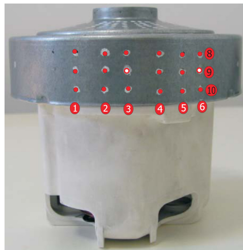
Fig. 7. Scheme of measured points on the cover's side surface (denser mesh)
