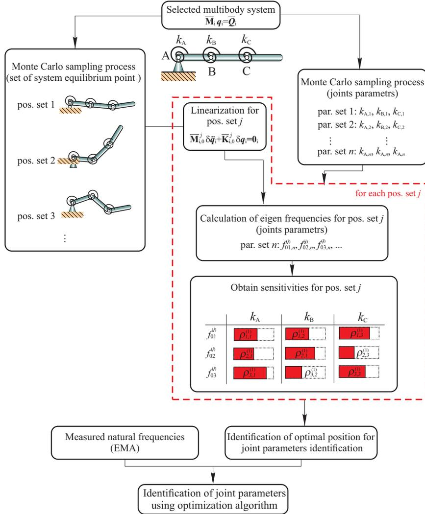
Figure 1: Schematic presentation of the multi-body parameter-identification algorithm.
