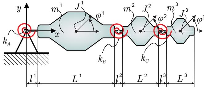
Figure 3: Multibody system under investigation.
