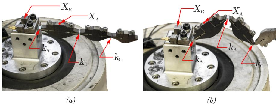
Figure 9: Experimental set-up used in the vibration test; (a) Configuration 1, (b) Configuration 2.
