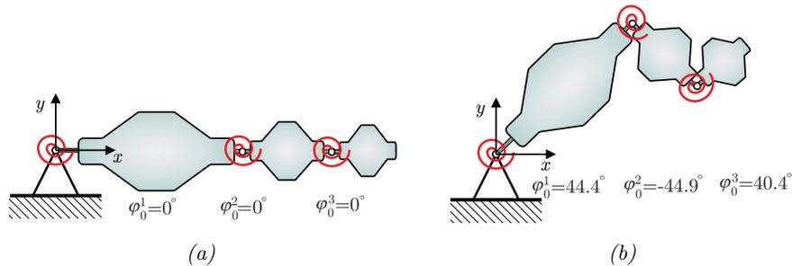
Figure 4: Analyzed configurations of the multi-body system; a) Configuration 1, b) Configuration 2.
