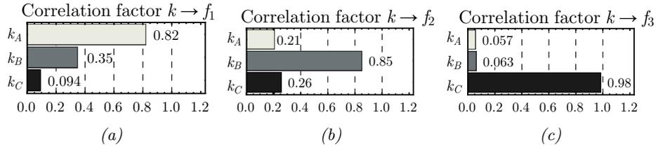
Figure 6: Interplay of joint-stiffness coefficients on the system's natural frequencies for Configuration 2; a) First natural frequency  $f_1$ , b) Second natural frequency  $f_2$ , c) Third natural frequency  $f_3$ .
