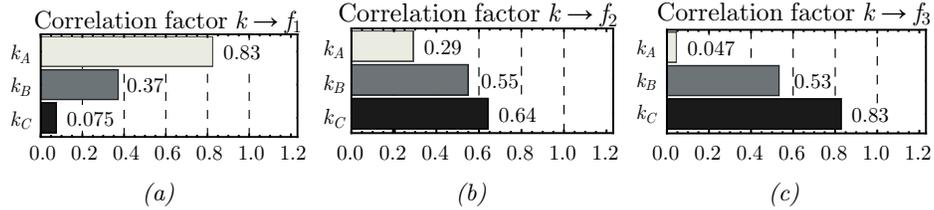
Figure 5: Interplay between the joint stiffness coefficients for the system's natural frequencies for Configuration 1; a) First natural frequency  $f_1$ , b) Second natural frequency  $f_2$ , c) Third natural frequency  $f_3$ .
