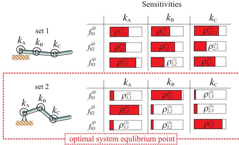
Figure 2: Identification of an optimal system equilibrium point for a multibody system.
