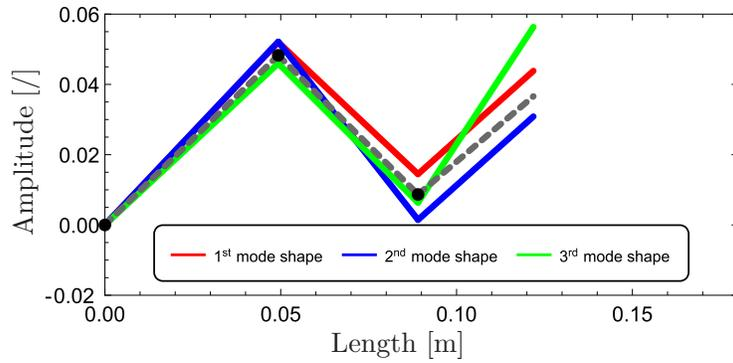
Figure 8: *The first three mode shapes for Configuration 2.*
