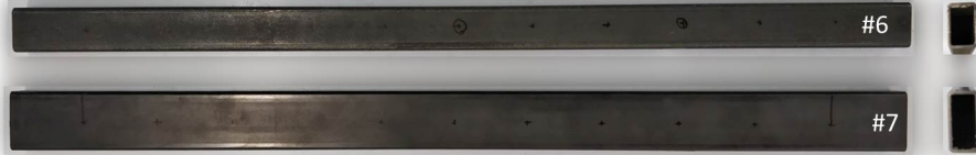
Figure 7: Laminated steel box beam
