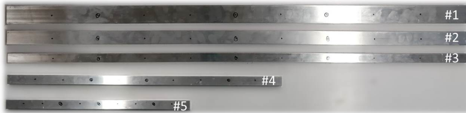
Figure 3: Aluminium beam specimens
